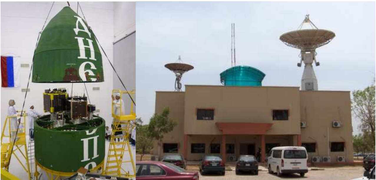
Figure 13 – NigeriaSat-2 integrated into Dnepr fairing (left) & NASRDA Abuja groundstation (right)
