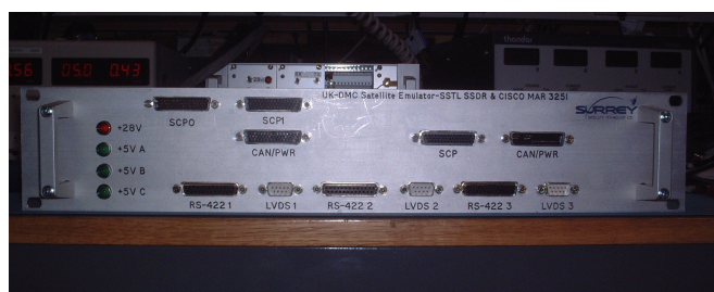
b. front view showing interface ports and flexible patchbay.
